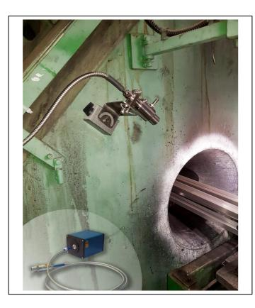
AST A5-EX-FO is a specially designed IR Pyrometer for noncontact temperature measurement of aluminum.
