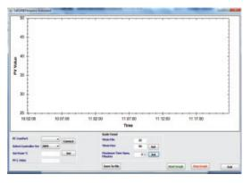
$\ddot{Y}$  CalSoft including for setting bath temperature and monitoring the PV. Graphical representations of PV/TIME with 2 hours data logging.
