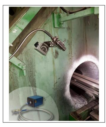
AST A5-EX-FO is a specially designed IR Pyrometer for noncontact temperature measurement of aluminum.
