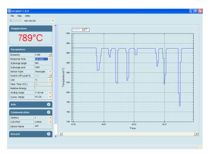
AST "Infrasoft" software is under standard scope of supply. It offers possibilities of parameter setting, view real time graph, offline graph and to evaluate measuring data. Communication between the pyrometer and the software is implemented via a cable connected between the pyrometer and the PC serial port.
