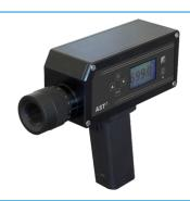
P390 is specially designed portable IR Pyrometer for non-contact temperature measurement of metallic surfaces and in flame heated furnaces i.e through flames and flue gas. At a wavelength of 3.9um, hot furnaces gases and clean burning gas flames are quite transparent and therefore permit temperature measurement of substances to be measured.
