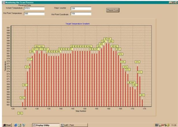
Figure 6 Profile temperature at the press exit
